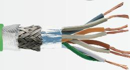
Suitable for flexible and protected installation in the interior for door control or in protecting tubes for outdoor laying at the bogie. Appropriate for light and medium mechanical stress. Certified acc. to EN 45545.
