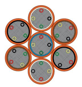
Application: Symmetrical cable with high flexibility. Minimum bending radius (easy to coil even in tight spaces) and high quality electrical performance (low voltage drop and low voltage unbalance). Can be used in long lengths.
