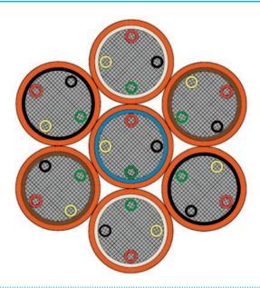
Application: Symmetrical construction with high flexibility. Minimum bending radius (easy to coil even in tight spaces) and high quality electrical performance (low voltage drop and low voltage unbalance). Can be used over longer distances.
