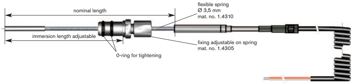
■ This dipstick resistance thermometer is especially appropriate to collect the temperature in engine oil. The dipstick can easily be inserted instead of the normal oil dipstick. The adjustable fixing tightens the opening so that during operation the oil cannot penetrate. With the help of the fixing, the immersion length of the dipstick can be modified.
