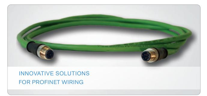
Application: For the field bus wiring of Profinet field bus systems in industrial sectors. This cable type is used for example in cable chain applications for automation and machine and plant construction with rough environments. The PUR outer sheath is resistant against rough environmental conditions.
